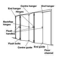
Foldaside projection butt hinges for frame to panel joints:
